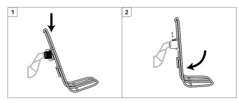
1. Align Upper Cross Bars of the Kanga Rack with the Upper Hooks of the KLICKfix Adapter.
